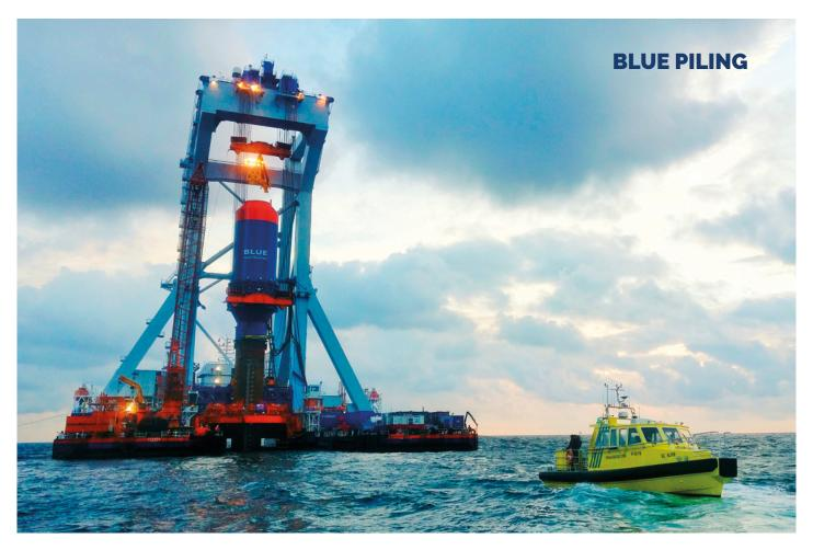
BLUE Piling Technology ™ (patent pending) uses the impact of a large (water) mass to drive down monopiles. The BLUE Piling blows aims at silent installation of the next generation monopiles. Unique BLUE Piling Technology features:
