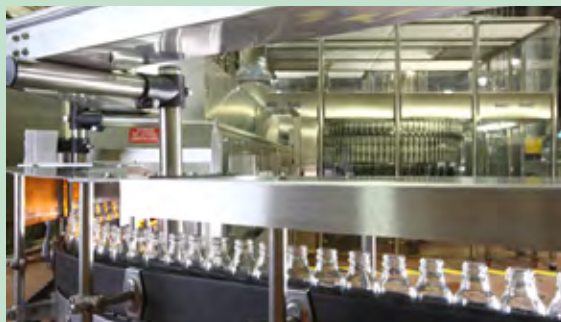
Figure: Pre-heating of glass bottles prior to filling. Source: Heraeus Noblelight GmbH, Infrared Process Technology
